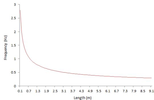
Fig. 2. 1<sup>st</sup> fundamental linear sloshing frequency (Hz) variation of a partially filled liquid 2D rectangular container in accordance with lateral length at  $h/l = 1.173$ .
