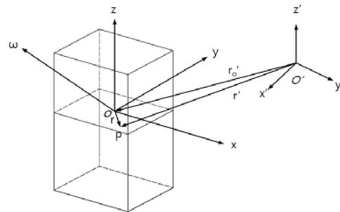
Fig. 1. Coordinate systems of a partially filled rectangular container.
