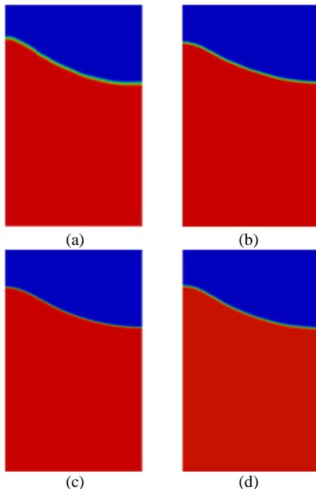
Fig. 3. Sloshed free surfaces of a partially filled rectangular container with adjusted 1<sup>st</sup> linear sloshing frequencies, (a) 1/4 scaled-down, (b) 1/2 scaled-down, (c) base, (d) 2 scaled-up.
