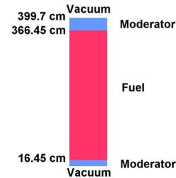
Figure 3. Axial configuration of simple 3D fuel assembly problem
