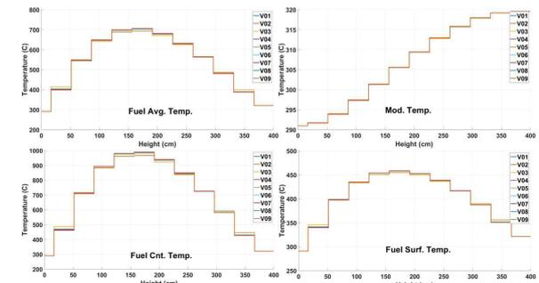
Figure 5. Axial temperature distributions for the simple 3D fuel assembly problem
