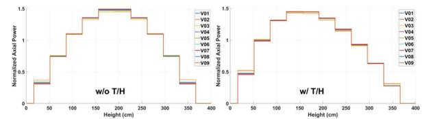
Figure 4. Axial power shape for the simple 3D fuel assembly problem
