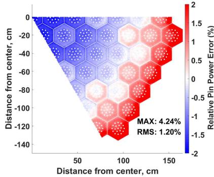
Figure 6. Relative pin power error distribution for the A04 V01 case
