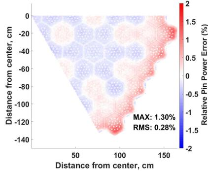
Figure 7. Relative pin power error distribution for the A04 V05 case
