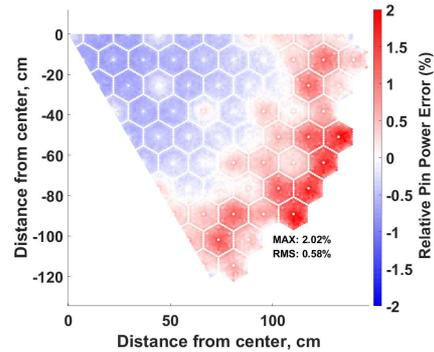
Figure 8. Relative pin power error distribution for the VVER-440 2D core problem
