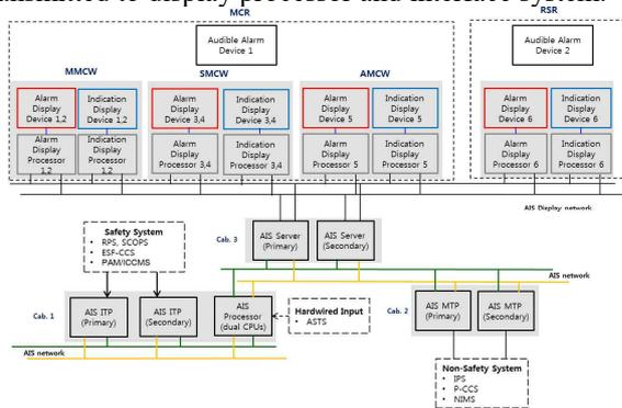
Fig. 1. System configuration of AIS.
