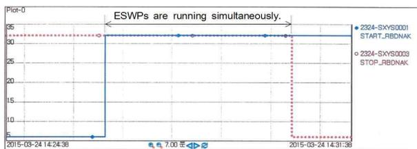
Fig. 3. The PI history of ESWPs' simultaneous running
