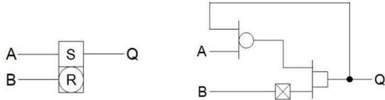
Fig. 5. Legend and configuration of the reset priority SR-latch
