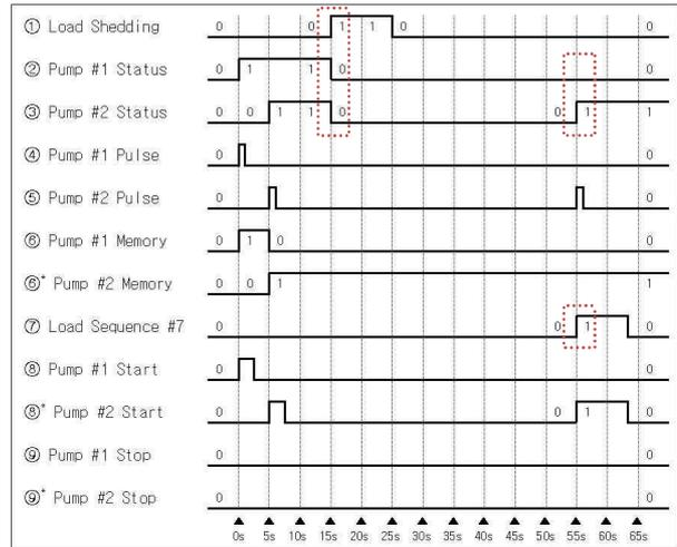
Fig. 7. Timing chart for the ESWP control signal in case of the LOOP during two ESWPs are running simultaneously in the train
