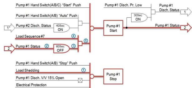
Fig. 1. The control logic for the ESWP
