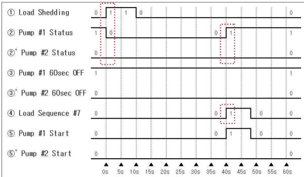
Fig. 2. Timing chart for the ESWP control signal in case of the LOOP during only one ESWP is running in the train
