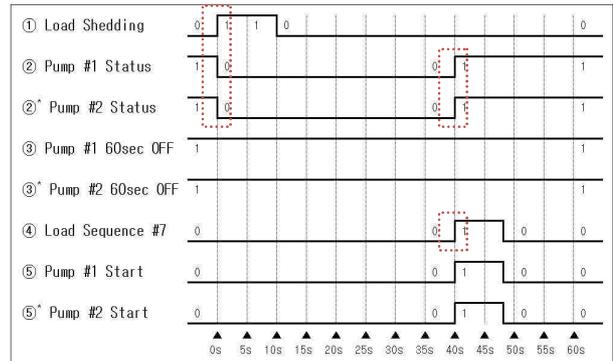
Fig. 4. Timing chart for the ESWP control signal in case of the LOOP during two ESWPs are running simultaneously in the train
