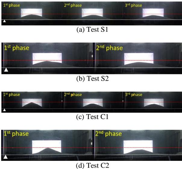
Fig. 4. Debris bed shapes at different phases
