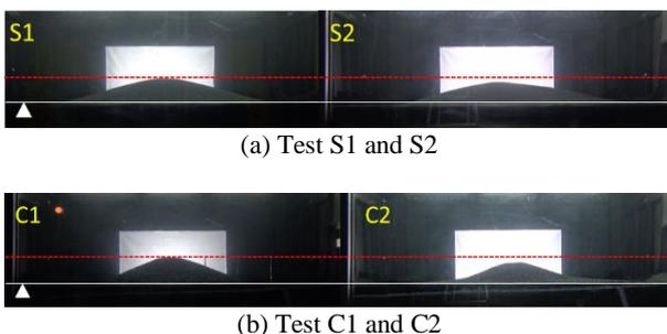
Fig. 6. Debris bed shapes at the end of the second phase
