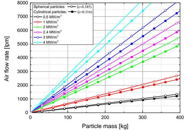
Fig. 3. Air flow rate for simulation of the steam generation according to decay heat and accumulated particle mass
