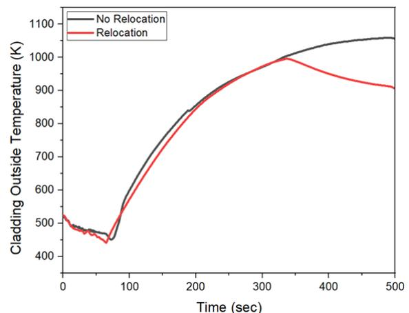
Fig. 3. A comparison of the cladding outside temperature during the 650.4 LOCA test at node 12 with and without the axial relocation model.
