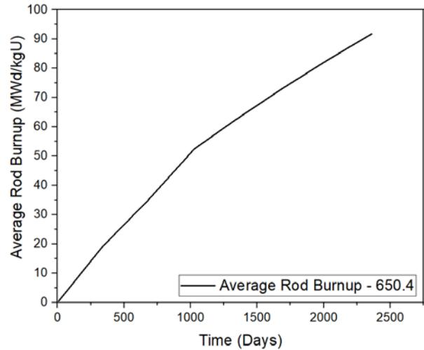
Fig. 2. Average fuel rod burnup obtained from FRAPCON-3.5
