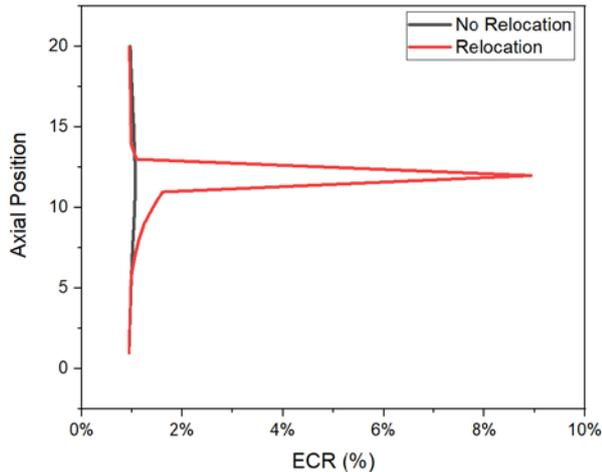
Fig. 4. A comparison of the equivalent cladding reacted (ECR %) during the 650.4 LOCA test 0.5 s after cladding failure with and without the axial relocation model.
