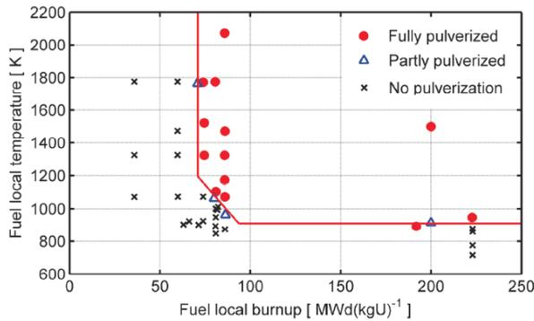
Fig. 1. Temperature threshold for pulverization in comparison with experimental data [3]
