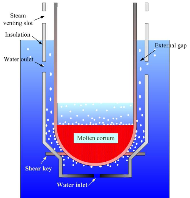
Fig.1 IVER-ERVC concept for SMART100
