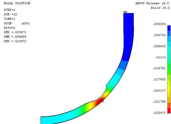
Fig. 3. ANSYS results on deformed geometry of lower reactor vessel wall by thermal and mechanical load under ERVC condition
