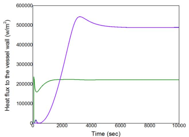
Fig. 2. Heat flux distribution from corium pool to the outer reactor vessel wall during IVR-ERVC
