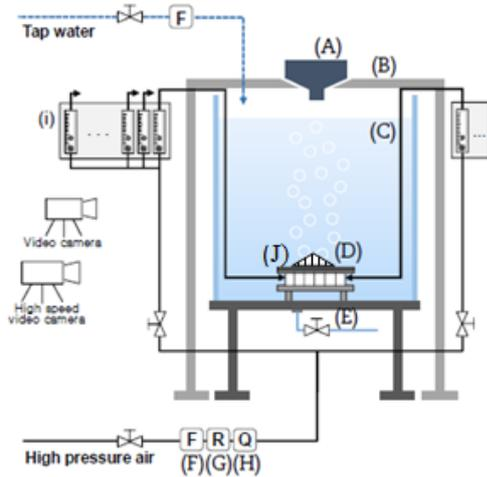
**Fig. 2:** Schematic diagram of DAVINCI test facility. (A) Funnel (B) Funnel rack (C) Test pool (D) Particle catcher plate (PCP) module (E) Water drain valve (F) Filter (G) Pressure regulator (H) Flowmeter (I) Rotameters with needle valves (J) bottom inclination mounting.
