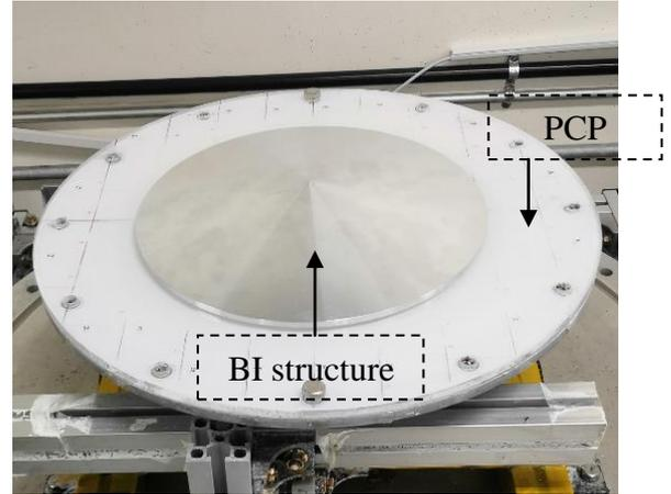
**Fig. 3:** Photographic view of bottom inclination mounting (BI) for QPC tests
