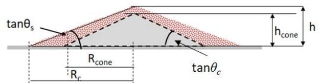
Fig. 6. A schematic diagram showing the side slope angle ( $\theta_s$ ) and characteristic length ( $R_c$ ) for a conical debris bed using bottom inclination structure ( $\theta_c$ )
