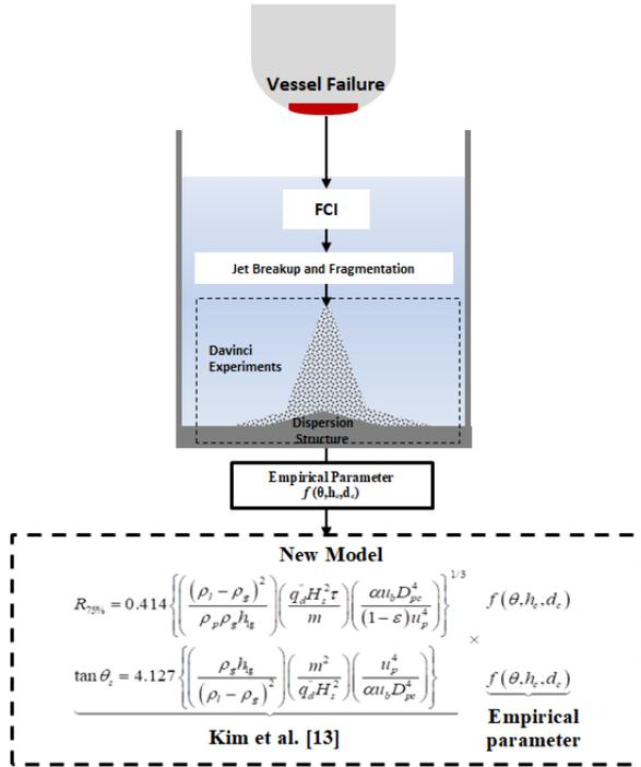
**Fig. 1:** Scope of the present study using DAVINCI tests with bottom inclination
