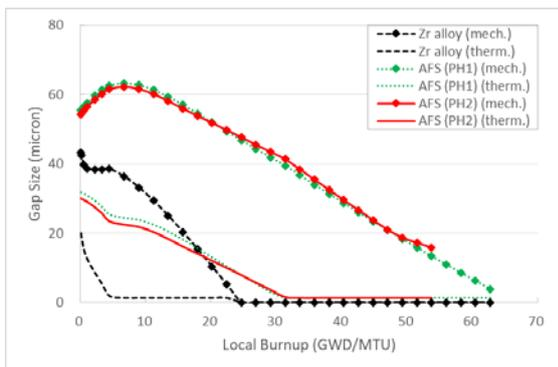
Fig. 3. AFS fuel mechanical and thermal gap between pellet and cladding vs. local burnup
