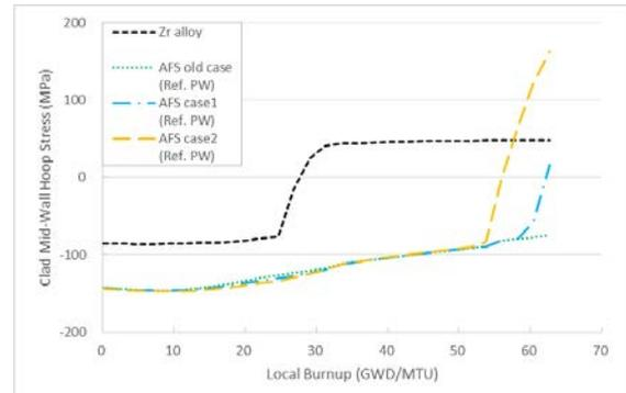
Fig. 7. Cladding mid-wall hoop stress for AFS with reference rod power history
