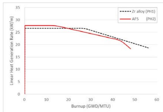
Fig. 1. Bounding power histories for Zr-based alloy cladding and AFS cladding fuel rods.
