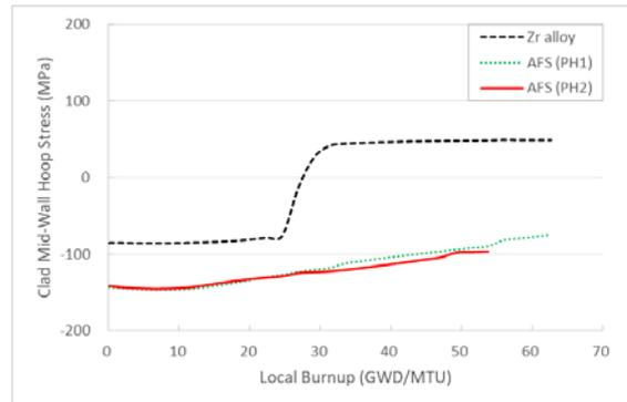
Fig. 4. AFS cladding mid-wall hoop stress vs. local burnup
