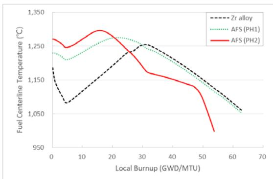
Fig. 2. AFS fuel centerline temperature vs. local burnup
