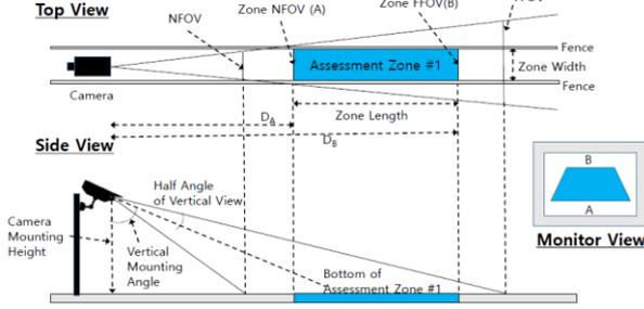
Fig. 2. Top and Side Views of Perimeter Assessment Zone Geometry
