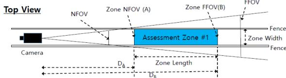
Fig. 1. Top View of Perimeter Assessment Zone Geometry
