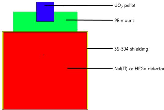
Fig. 1. Simplified detector geometry
