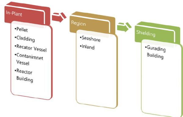
Fig. 2. Another barrier system for multiple-barrier in nuclear safety.
