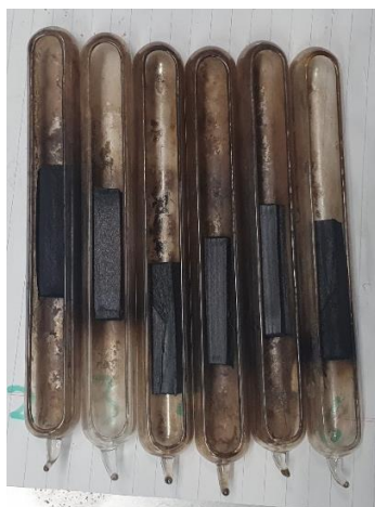
Fig. 3. The wood sample by incomplete combustion
