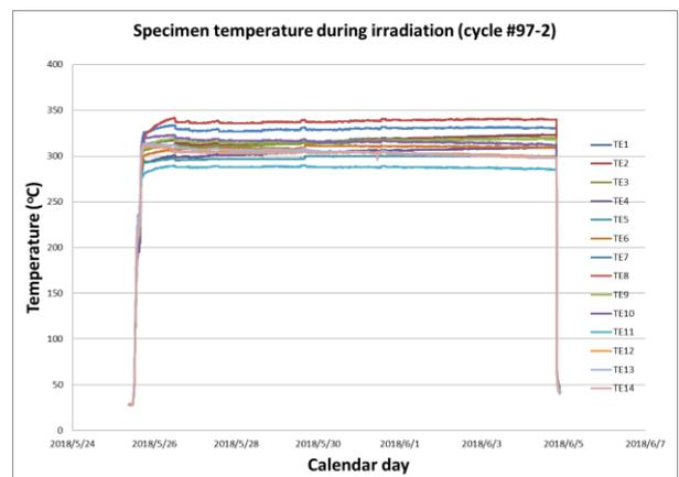
Fig. 2. Measured temperatures during the ARAA testing
