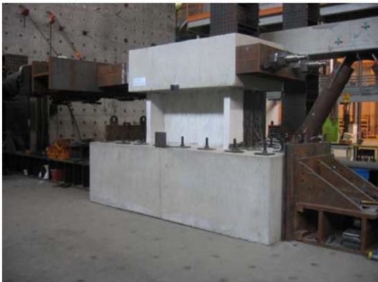
Fig. 4. Test setup for cyclic test of SC shear wall
