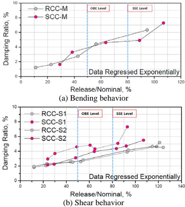
Fig. 3. Damping ratios from test data regression
