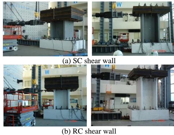
Fig. 1. Test setup for free vibration test
