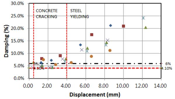
Fig. 6. Damping distribution dependent on lateral displacement of SC shear walls
