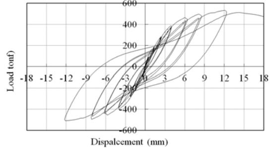
Fig. 5. Typical test result for cyclic test of SC shear Wall
