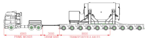
Fig. 2. Schematic drawing of trailer to be used in road test
