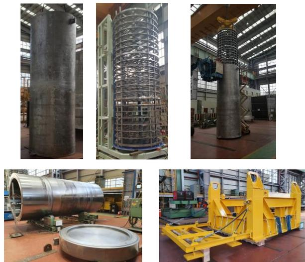
Fig. 1. Test model fabrication (a) canister (b) internal structure (c) installation of disks into canister (d) cask (e) cradle.
