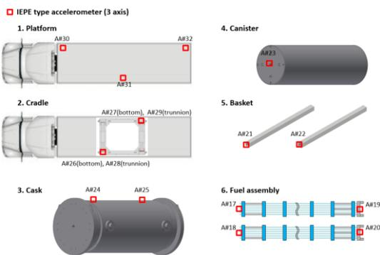
Fig. 4. Data acquisition system diagram.
