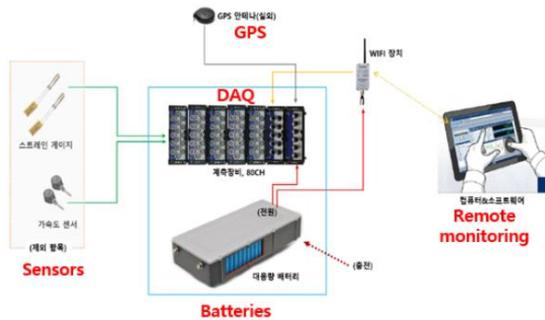
Fig. 3. Data acquisition system diagram.
