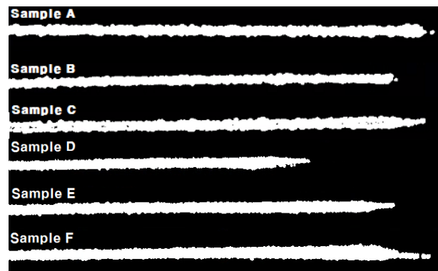
Figure 1. Visualized thickness distribution of the fuel meat part in the fabricated samples
