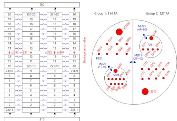
Fig. 1. Hydraulic channels and fuel rods
