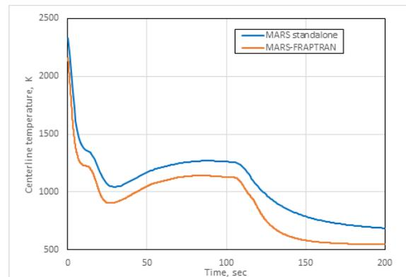
Fig. 4. Comparison of fuel centerline temperatures
