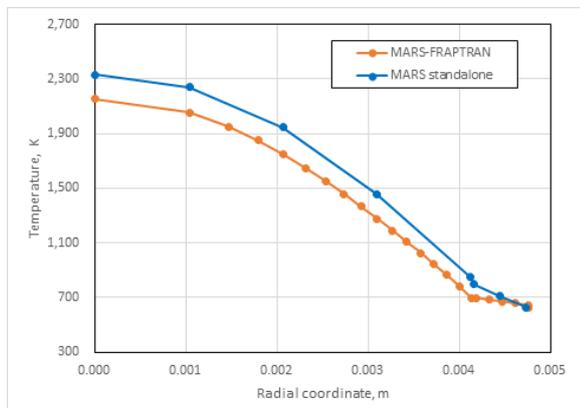
Fig. 6. Comparison of temperature distribution within the fuel at the beginning of transient
