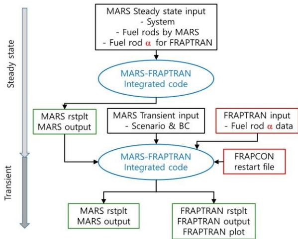
Fig. 2. Overall process for MARS-FRAPTRAN calculation
