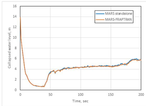
Fig. 5. Comparison of collapsed water level of hot channel
