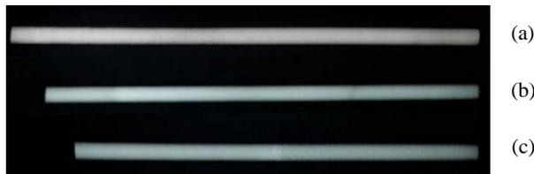
Fig. 2. X-ray radiography of the simulated sphere-packed fuel rods; (a) filling of pre-mixed power, (b) infiltration filling after parallel filling, (c) continuous infiltration filling.
