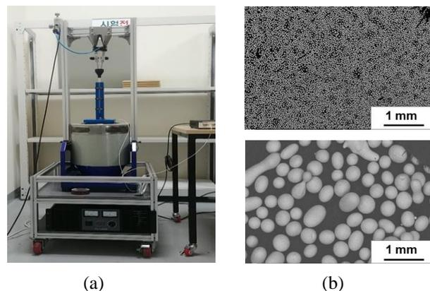
Fig. 1. Frequency-variable vibration packing system (a), spherical SUS 316L metal powder (upper part: < 325mesh, lower part: < 50mesh) (b).
