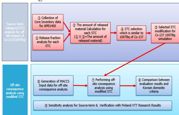
Fig. 1. Research Framework for Verification of ‘Cs-137 requirement’
