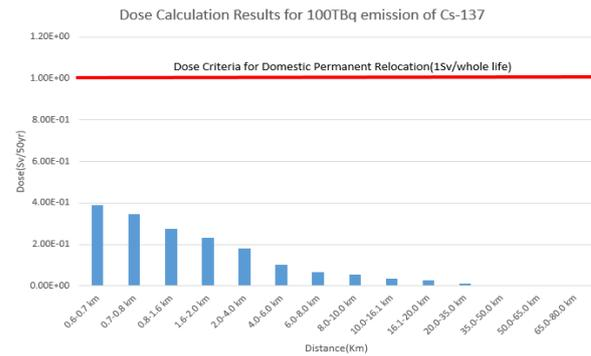
Fig.3. Dose Calculation Results for Cs-137 100TBq
