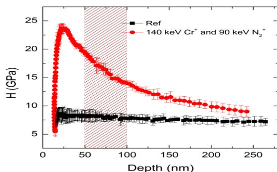
Fig. 3. Nano-indentation result before and after ion implantation
