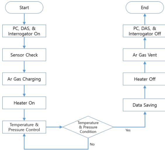
Fig. 3. Test procedure
