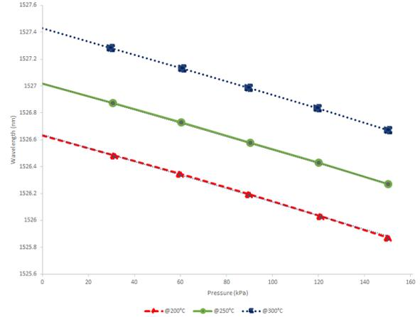
Fig. 4. Wavelength of FBG for system pressure measurement including temperature induced wavelength shift at each temperature
