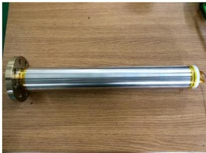
Fig. 1. The prototype of FBG-based pressure transmitter
