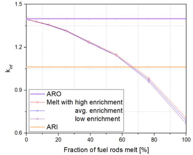
Fig. 3. Sensitivity of the criticality on the various enrichment of the fuel melt (Case 1)
