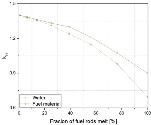
Fig. 5. Sensitivity of the criticality on the type of materials in the parts of the rods degraded (Case 3)
