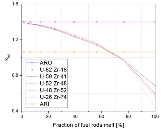
Fig. 4. Sensitivity of the criticality on the various fractions of U and Zr (Case 2)
