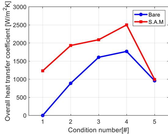
Fig. 4. Average values of heat transfer coefficient of copper condenser tubes
