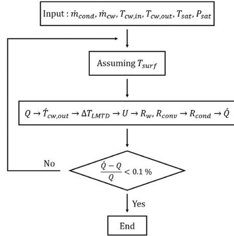
Fig. 3. Iteration programming flowchart [1]
