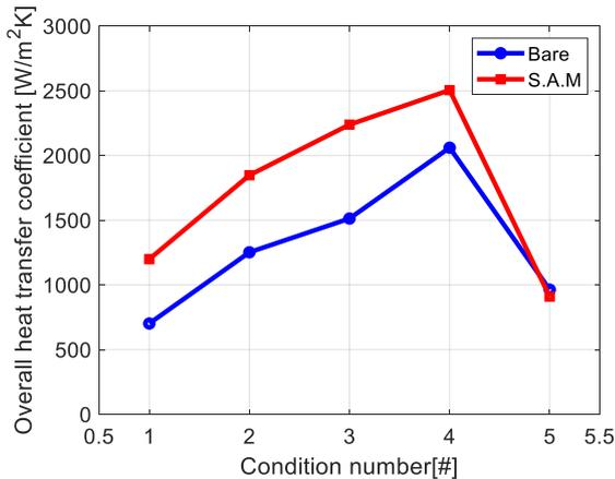
Fig. 5. Average values of heat transfer coefficient of SUS condenser tubes
