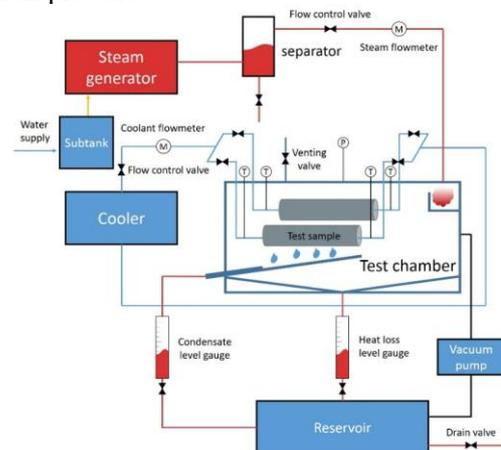
Fig. 2. Schematic Diagram of Experimental Facility
