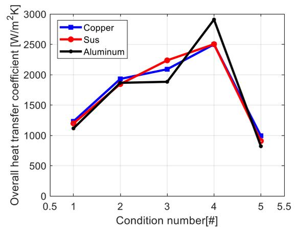
Fig. 6. Overall heat transfer coefficient comparison among copper, SUS, and aluminum S.A.M tubes
