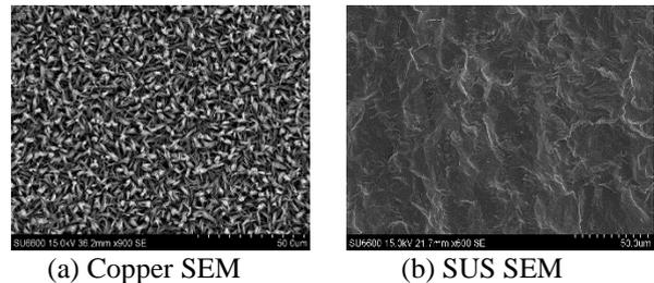
Fig. 1. SEM images of S.A.M modified surfaces
