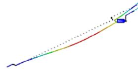
Fig. 2. 1<sup>st</sup> Mode shape of the piping system (2.0 Hz)
