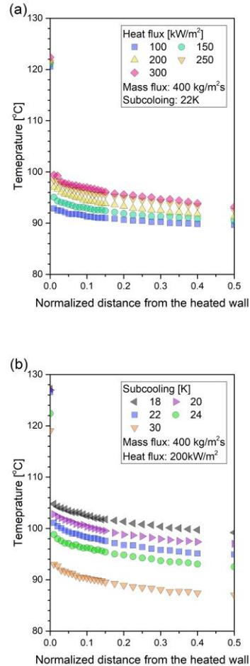
Figure 3. Wall and fluid temperature with varying heat flux (a) and inlet subcooling (b)
