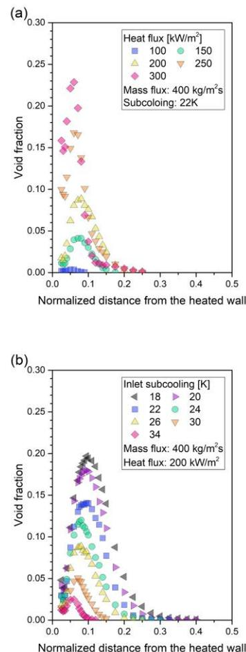
Figure 1. Void fraction with varying heat flux (a) and inlet subcooling (b) [1]
