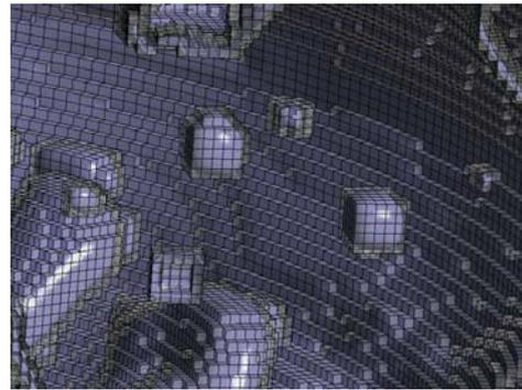
Fig. 4. Identification of melt drops and their sizes
