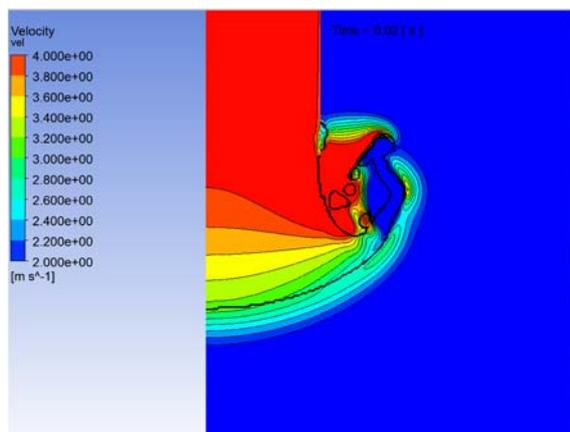
Fig. 3. Velocity magnitude near the jet leading edge ( $V_{jet} = 4.0$  m/s, dark solid line: melt interface)
