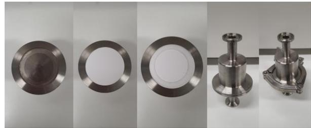
Figure 4. Filter Assembly Order
