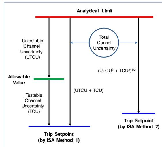
Fig. 1. ISA RP67.04 trip setpoint determination methods for rising trip parameter
