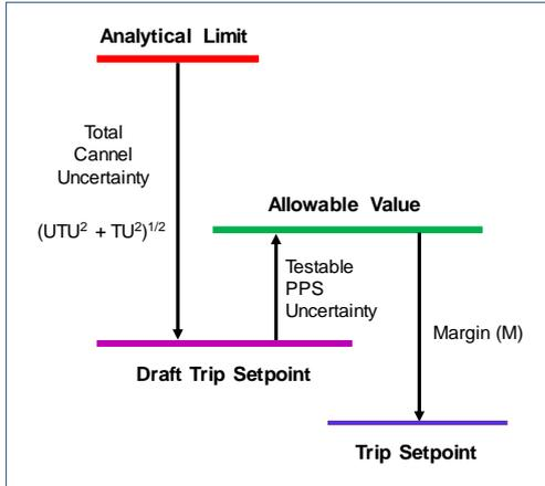
Fig. 2. APR1400 trip setpoint determination method for rising trip parameter
