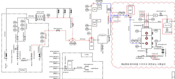
Fig.2. Schematic diagram of ISLOCA Aerosol Pool Scrubbing Test Facility
