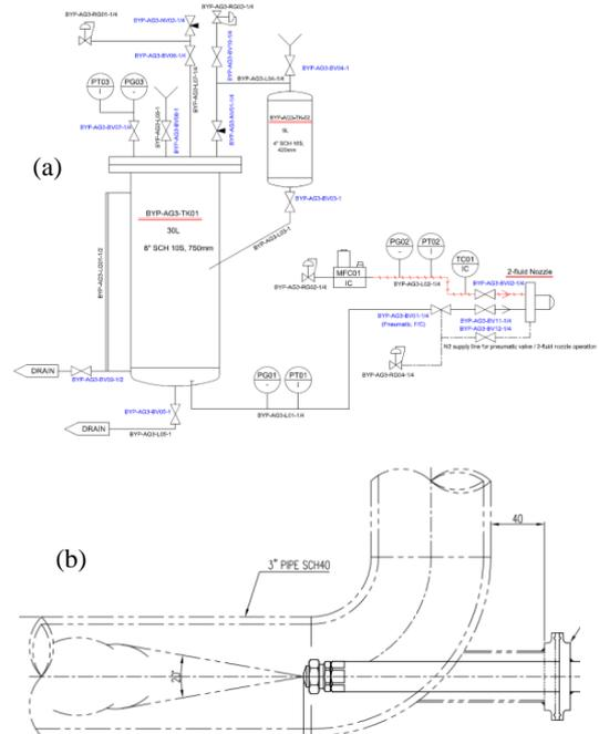
Fig. 4. Schematic diagram of Aerosol Generation/Injection System; (a) Aerosol Generation System; (b) Aerosol Injection
