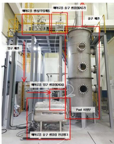
Fig.3. Configuration of ISLOCA Aerosol Pool Scrubbing Test Facility
