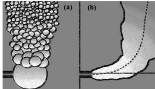
Fig.1. Schematic view of the two conceptual flow regime; (a) Globular Regime; (b)Jet Injection Regime[1]
