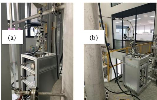
Fig. 6. Configuration of Aerosol Sampling System; (a) Inlet of the pool; (b) Outlet of the pool
