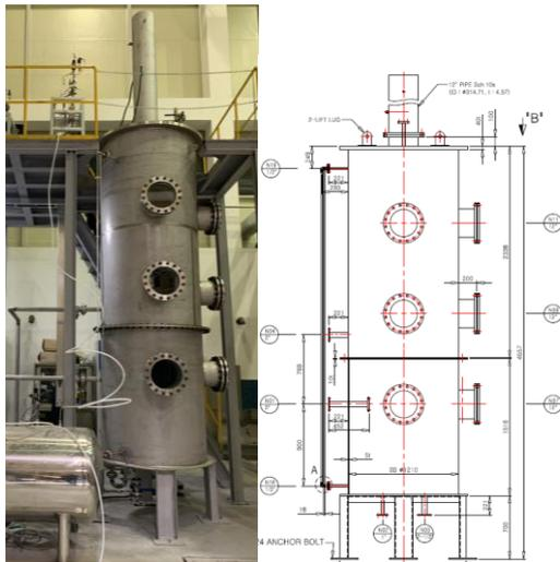
Fig. 5. Pool Configuration of the test facility
