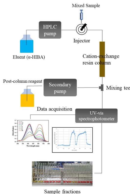
Fig. 1. Photographs for LC system with the post-column detection.
