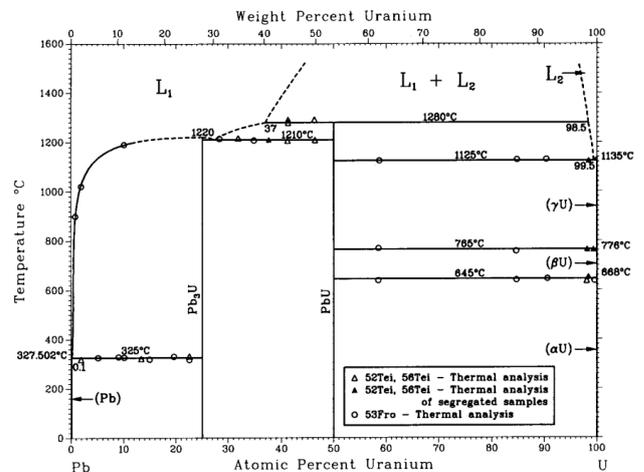
Fig. 4. Phase diagram of U-Pb system [8]
