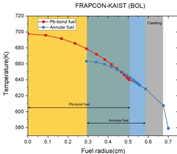
Fig. 5. Radial temperature calculation comparison results
