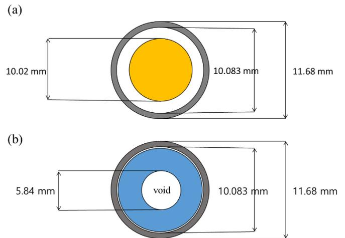
Fig. 1. Schematic cross section image of fuel rod (a) Pb-bond fuel (b) annular fuel
