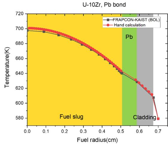
Fig. 3. Radial temperature calculation results with lead bond
