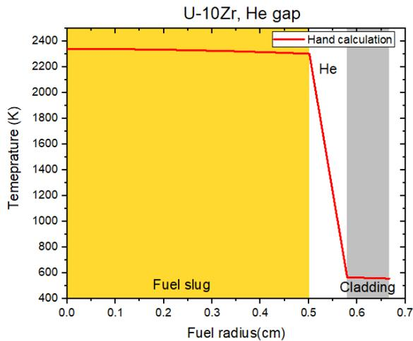
Fig. 2. Radial temperature calculation results by hand calculation with the helium gap
