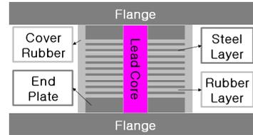
Fig. 1 Cross-Sectional Shape of the LRB
