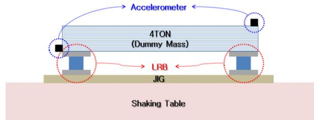
Fig. 2 Schematic Diagram of 3D Shaking Table Test
