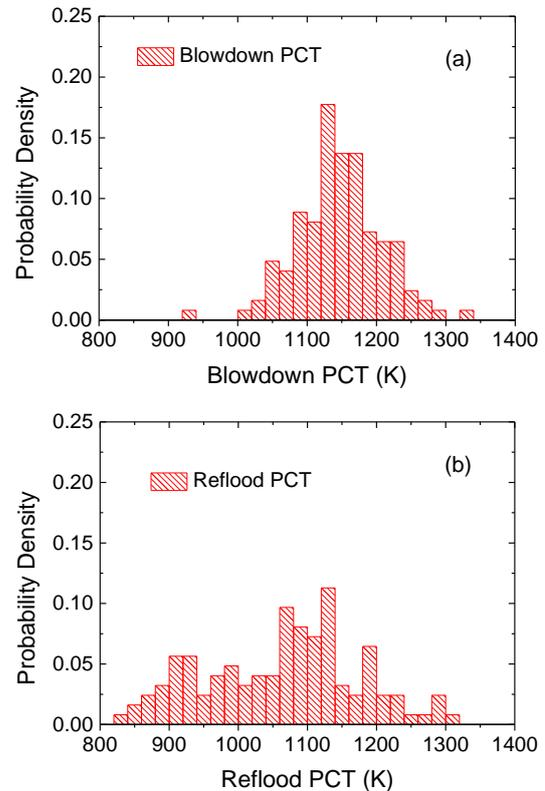
Fig. 1. PCT distributions; (a) blowdown phase (b) reflood phase
