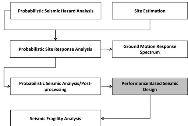
Fig. 1. Procedure of probabilistic seismic design
