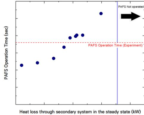
Fig. 3. Comparison of PAFS operation time according to heat loss through the secondary system
