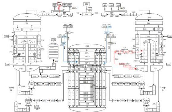
Fig. 1. SPACE Nodalization of the ATLAS facility
