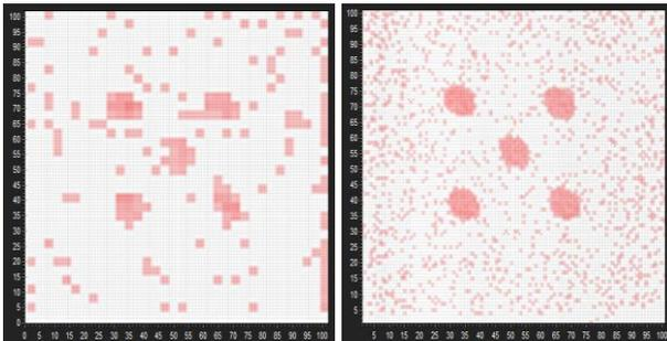
Fig. 4. 2D distribution of uranium in a point distributed swipe measured by coarse mode (left) and fine mode (right)
