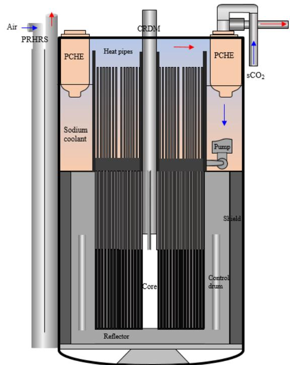
Fig. 2. Schematics of H-MMR core. PCHE, printed circuit heat exchanger; PRHRS, passive residual heat removal system, CRDM, control rod drive mechanism.
