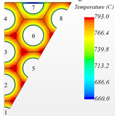
Fig. 5. Contour plot of temperature in the fuel assembly when the core height is 0.6m.
