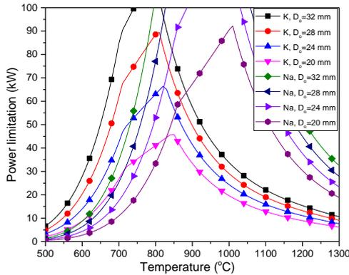
Fig. 3. Operating limits as a function of operating temperature for potassium and sodium heat pipe with a diameter of  $D_o$  and annular wick structure.
