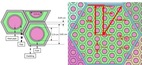
Fig. 4. Specific design parameters for the H-MMR core.
