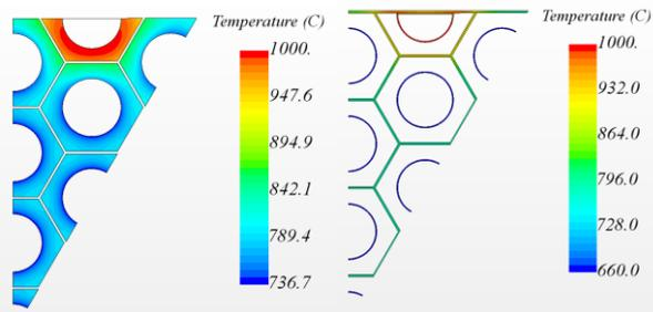
Fig.7. Contour plot of temperature in the fuel assembly for the failure of number 7 heat pipe
