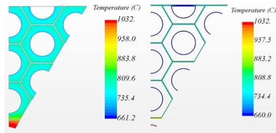
Fig.6. Contour plot of temperature in the fuel assembly for the failure of number 1 heat pipe.
