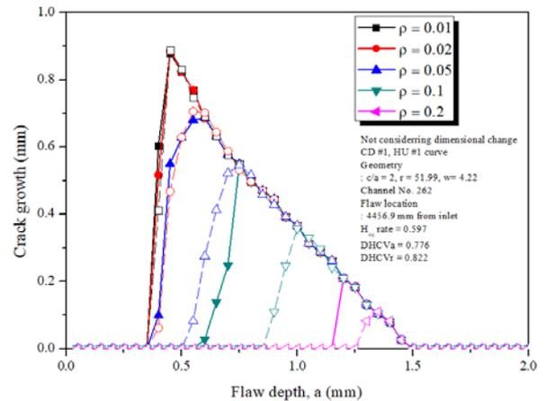
Fig. 7. Crack growth evaluation by DHC.
