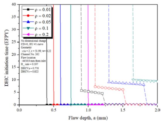
Fig. 6. Crack initiation time by DHC.
