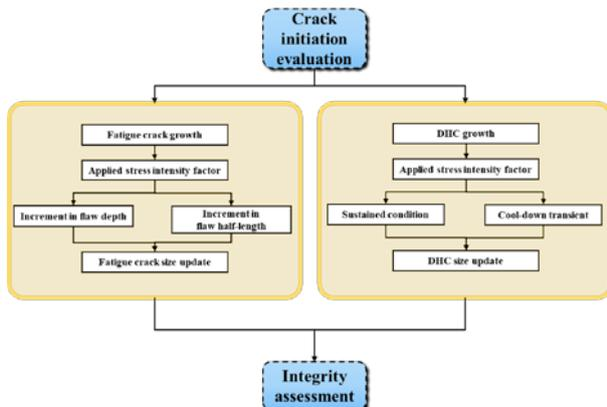
Fig. 4. Evaluation of crack growth.
