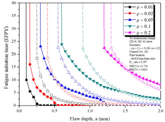
Fig. 5. Crack initiation time by fatigue.
