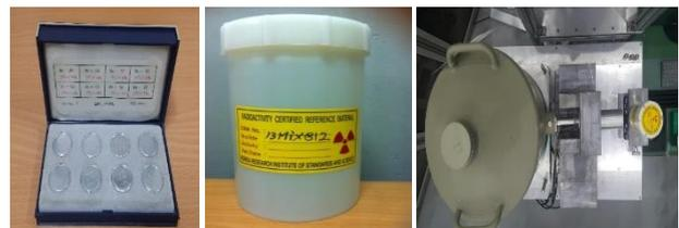
Fig. 2. Standard sources (point: left, volume: middle) and Measurement environment (right).
