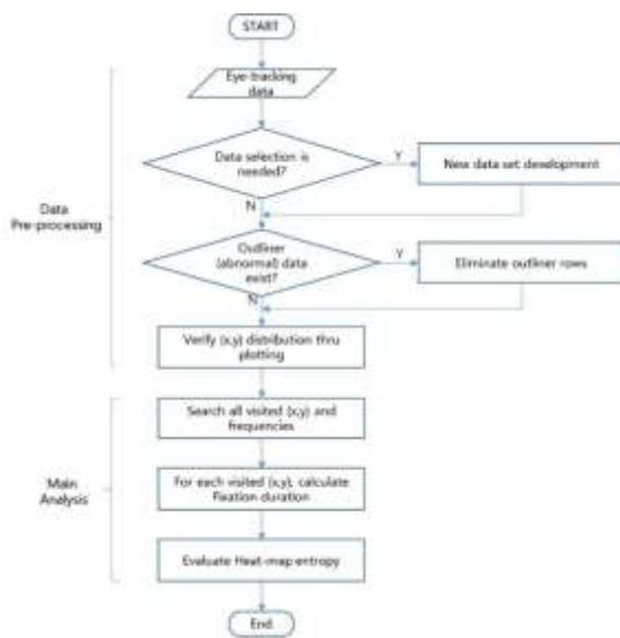
Fig. 2. Flow chart for the heat-map entropy evaluation program
