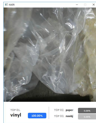
Fig. 3. A result of radioactive waste classification by computer vision-based system
