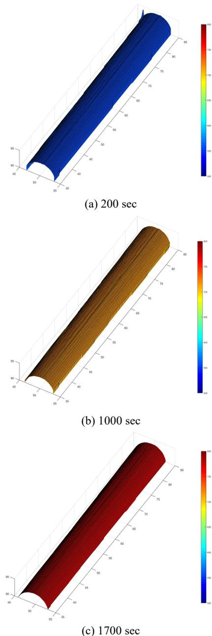
Fig. 8. Clad geometry and surface temperature during reflow test
