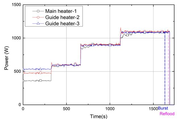
Fig. 9. Applied electric power during burst test
