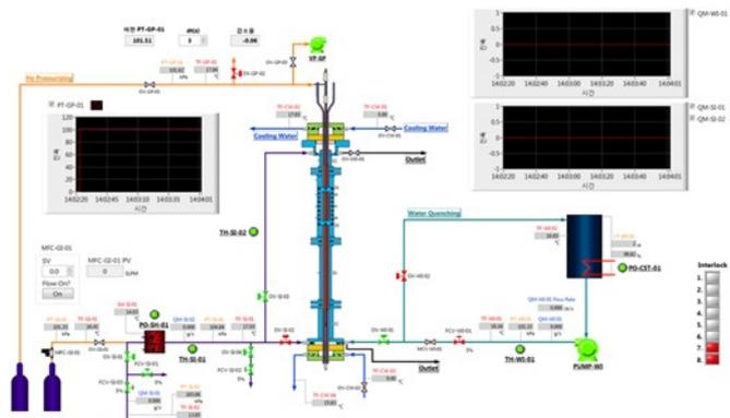
Fig. 4. Control panel for fluids supply system.
