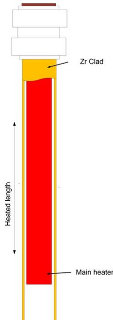
Fig. 3. Assembled heater and cladding
