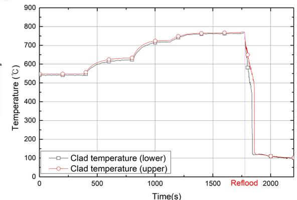
Fig. 6. Clad temperature during reflood test
