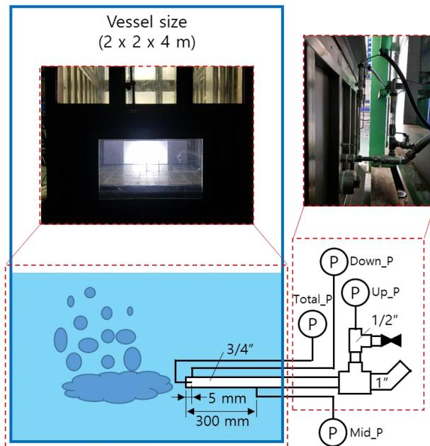
Figure 1 Schematics of preliminary test facility
