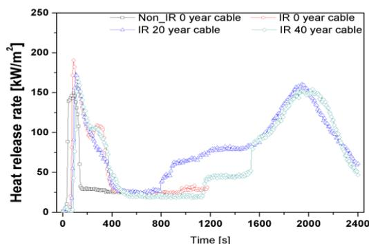
Fig. 1. HRR curves with respect to time for specimens
