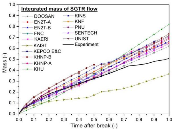
Fig. 4. Integrated mass of break flow from SGTR
