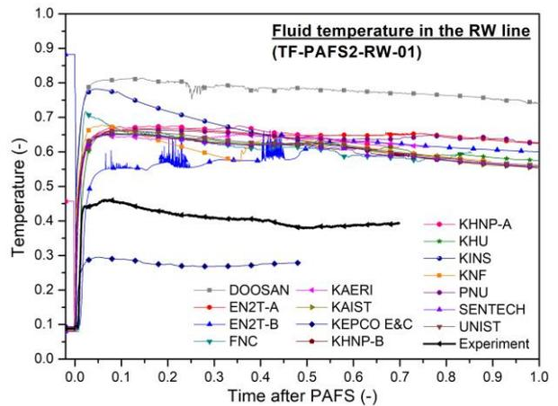
Fig. 7. Fluid temperature in RW line of PAFS
