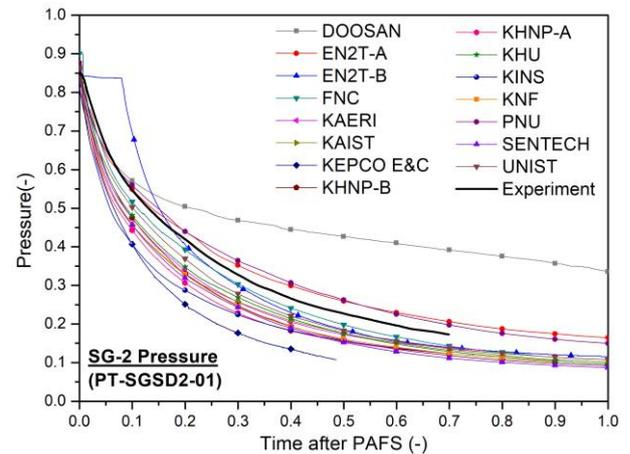
Fig. 3. Secondary system pressure behavior after
