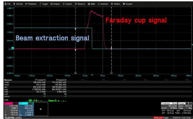
Fig. 4. A timing between the TTL signal from beam extraction (blue) and charge collection from faraday cup (red) on oscilloscope
