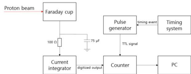
Fig. 1. The configuration of beam current measurement system.
