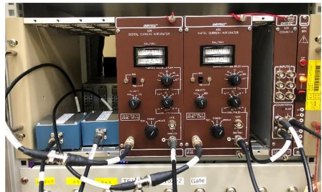
Fig. 2. Installed current integrator, storage element, and counter.
