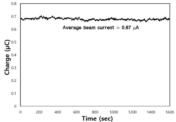
Fig. 5. The acquired charge per pulse data for 1600 sec under beam repetition rate of 1Hz.
