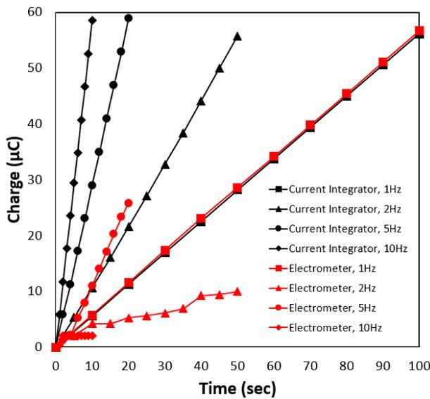
Fig. 3. Linearity of charge accumulation using current integrator and electrometer under 1Hz, 2Hz, 5Hz, and 10Hz
