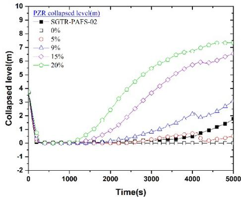
Fig. 2. Pressurizer level behavior in case of different heat loss on pressurizer
