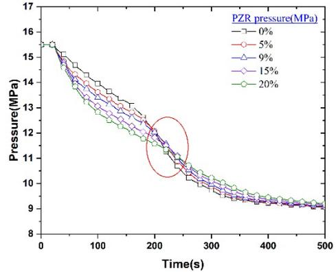
Fig. 4. Pressure in pressurizer by calculation results.
