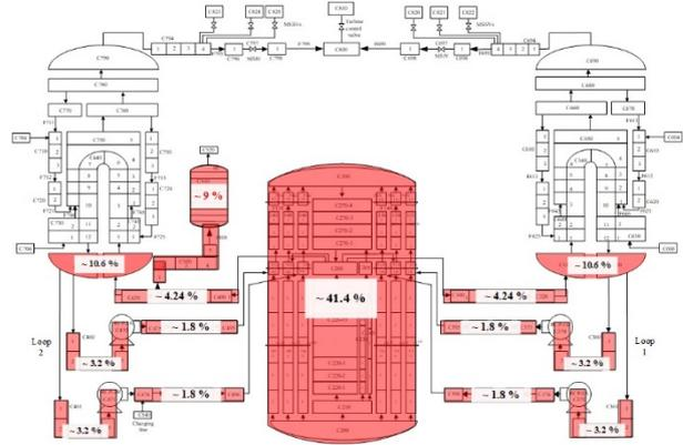
Fig. 1. Example illustration of heat loss proportion modeled in 1-C case for sensitivity analysis.
