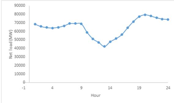
Fig. 1. Net electricity load demand
