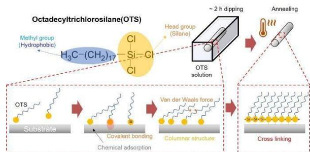
Fig.1 A schematic for fabrication of OTS monolayer coatings on the substrates.
