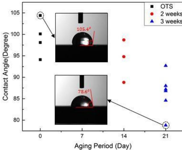
Fig.2 Contact angle dependings on the aging period in OTS coating,
