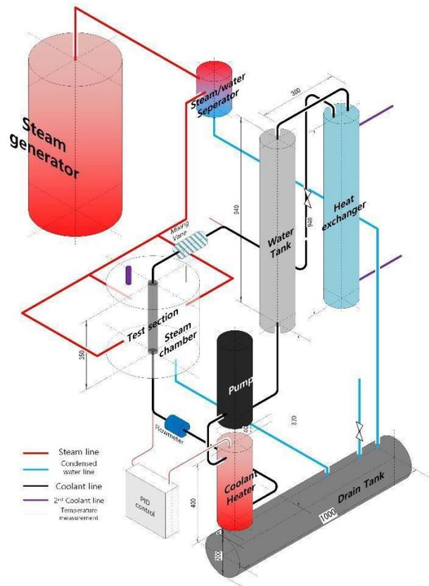
Fig.3 Schematic of condensation heat transfer experiment system.
