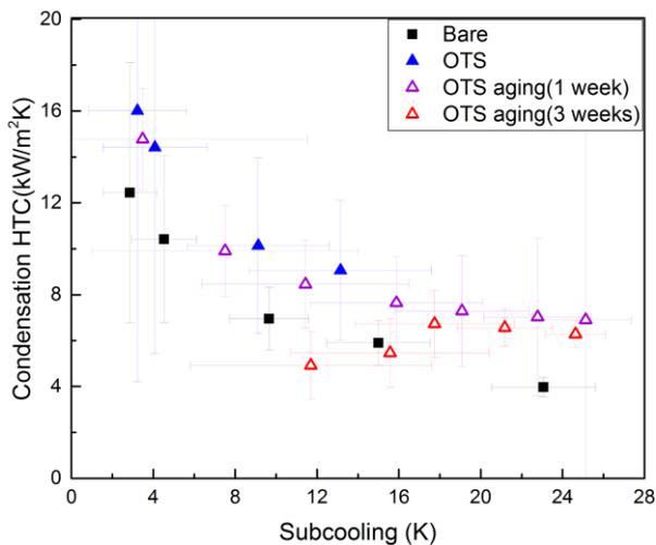
Fig.5 Condensation heat transfer of each surface with aging effect
