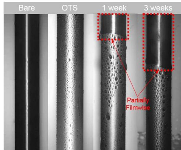
Fig.4 Visualization of the condensation on each surface.
